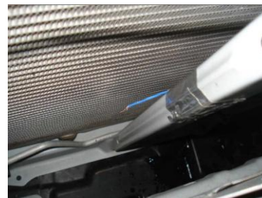
Figure 4: The inlet and outlet air temperature sensors of fan on the vehicle
